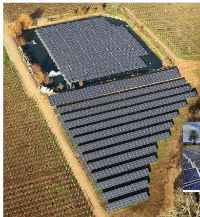
• Land based and floating solar panels at a vineyard in Oakville, CA $8,805/kW e
